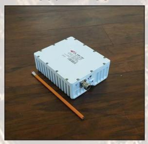
This smallest and lightest 2W L-To C-Band Block Up Converter is based on GaN technology. High power efficiency resulting in the low current (<1.17 amps @ 24VDC). The unit covers Standard (5.85-6.425 GHz) C-Band frequencies.
