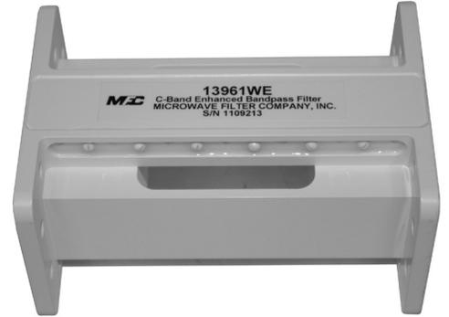
Utilizing a durable and true one piece body/flange construction, the 13961WE is shipped with hardware & gasketing and is ready to install between the feedhorn and the LNB/LNA.
