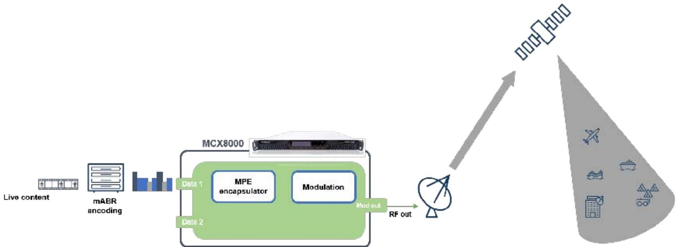
The benefits of broadcasting over satellite networks for content distribution are well known for scale and quality of experience. Now broadcasters can leverage multicast to expand their portfolio to include IP-based video content models, including OTT. Designed for the future of broadcasting, the MCX8000 is a DVB Native IP compliant solution capable of efficiently multicasting OTT content over satellite with IP encapsulation rates of over 300 Mbps across multiple carriers.
