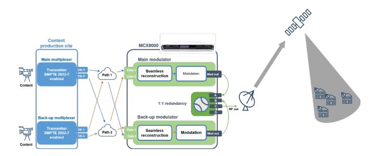
The MCX8000 Multi-Carrier Satellite Gateway has the right features for squeezing the maximum throughput out of the available bandwidth, whether using the DVB-S, DVB-S2, or DVB-S2X standard. It supports SMPTE 2022-7 Seamless Protection Switching providing reliable transport stream delivery.
