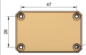
4x LID SCREW HOLES DRILLED THOROUGH & TAPPED M3x0.5mm TO 10mm DEPTH FOR MOUNTING UNIT
