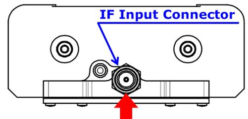
Connect the coaxial cable, and supplied the DC Power and 10MHz reference signal from modem.
