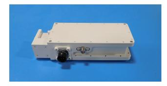
LKKC-20120 Ka-Band Ultra Low Noise Amplifier is specially designed for satellite earth station and other telecommunications applications. Utilizing state-of-the-art HEMT and GaAs MMIC technology, this amplifier has been designed for both fixed and transportable applications. The noise temperature specification is guaranteed over the full bandwidth of the LNA, and measured using a cryogenic hot/ cold load test setup.
