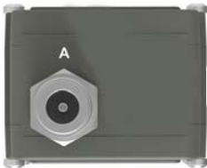
Connector A (standard) Type: N female, (option F female or SMA female) Functions: L-Band out, DC in, External 10 MHz in
