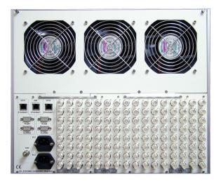
Vortex can be part populated in blocks of 16 inputs or outputs for smaller matrices and then hot expanded as your routing requirements change.
