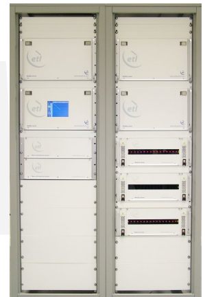
64 x 64 Enigma system with splitters & combiners
