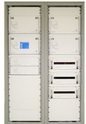
64 x 64 Enigma system with splitters & combiners
