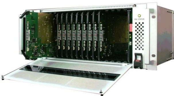
Front view showing hot-swap RF Module
